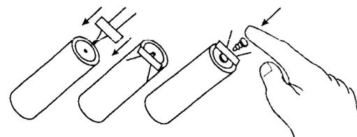
**11** Select a A8-3 engine for your first launch. This will give you an approximate altitude of 300 to 400 feet (152 - 213 m). Carefully insert igniter into engine and bend igniter. Use an erigine plug or masking tape to secure igniter in place.
