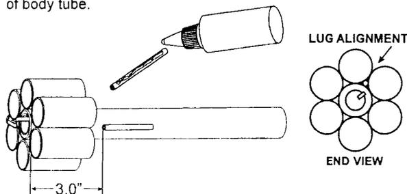
**5** Measure 3" from end of rocket. Make a mark with pencil so that it is between tubes as shown above. Apply a drop of white glue to launch lug and spread it out with your index finger. Glue launch lug to body tube at 3" mark. Lug needs to line up with joint between tubes.
