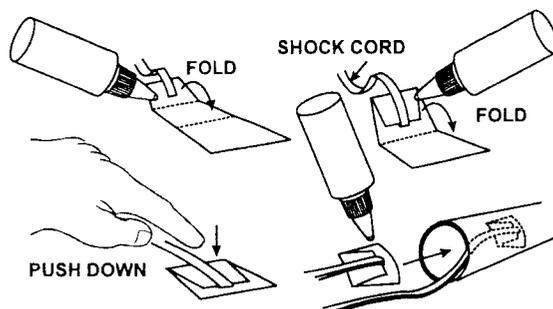
**4** Cut shock cord mount (Part N) from front of instruction sheet. Locate shock cord (Part J). Apply a drop of glue to number one and put end of shock cord into glue. Fold number one into number two, then apply glue to back of number one. Fold number two into number three. Squeeze the mount between your fingers until glue starts to set. When mount is dry, apply two drops glue to side that has Custom logo. Insert mount at least 1.5" into end of body tube.
