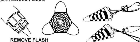
**6** Cut out the parachute with scissors. Assemble parachute using instructions provided with parachute. With a pencil or pen, clear away flash from both eyelets on nose cone. Pass shroud lines through one of eyelets on nose cone. Slide nose cone through loop in shroud line and pull tight.
