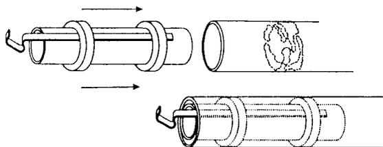
**2** The glue on joints of rings should be completely dry before starting this step. Apply white glue to inside of body tube (Part A). Glue should be about one inch inside end of tube. Insert engine mount into body tube with one swift and even motion. **DON'T STOP UNTIL BOTH TUBES ARE EVEN!**
