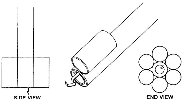
**3** Apply white glue to one of tube fins. Glue should run length of tube fin. Glue tube fin to end of body tube that has engine mount installed. Both tubes should be even. Continue gluing tube fins until all 6 tube fins have been glued.
