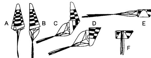
A - Pull parachute to form a spike. D - Fold top part to bottom.
