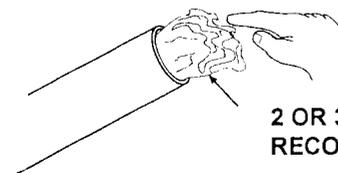
**9** To protect parachute from hot exhaust which can melt the plastic, recovery wadding must be used. loosely insert 2 or 3 squares into body tube. Fold parachute as in step 10, and then insert parachute. Place nose cone back into tube. Your rocket is now ready to launch.
