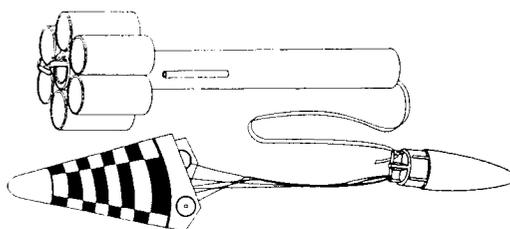
**7** Tie end of shock cord to other eyelet on nose cone.
