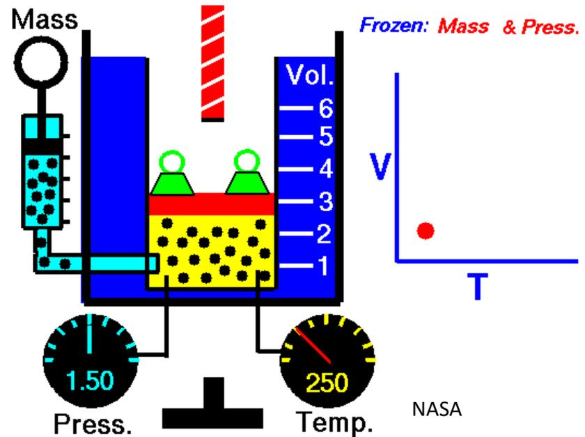
$$\frac{V_1}{T_1} = \frac{V_2}{T_2}$$
