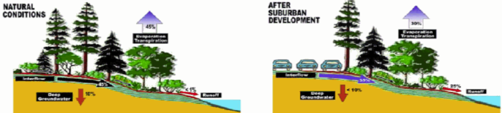
Fig. 3.21 – Relationship between impervious cover and surface runoff. Impervious cover in a watershed results in increased surface runoff. As little as 10 percent impervious cover in a watershed can result in stream degradation. In Stream Corridor Restoration: Principles, Processes, and Practices (1998). By the Federal Interagency Stream Restoration Working Group (FISRWG) (15 Federal agencies of the U.S.)
